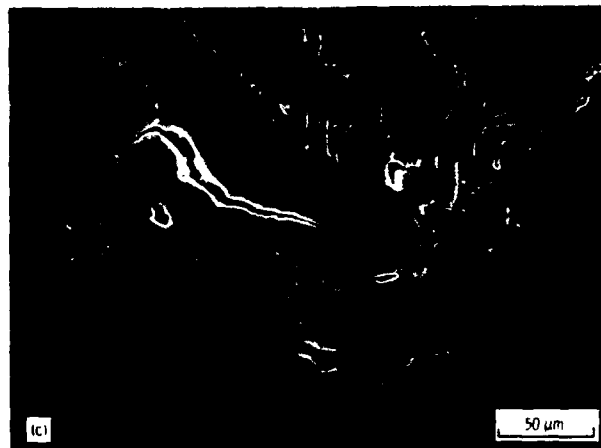
(a) Section through fracture surface (specimen HH-57, N_f = 25 ). (b) Surface-initiated intergranular crack (specimen HH-61, N_f = 117 ). (c) Internal grain boundary cracks (specimen HH-61, N_f = 117 ).
