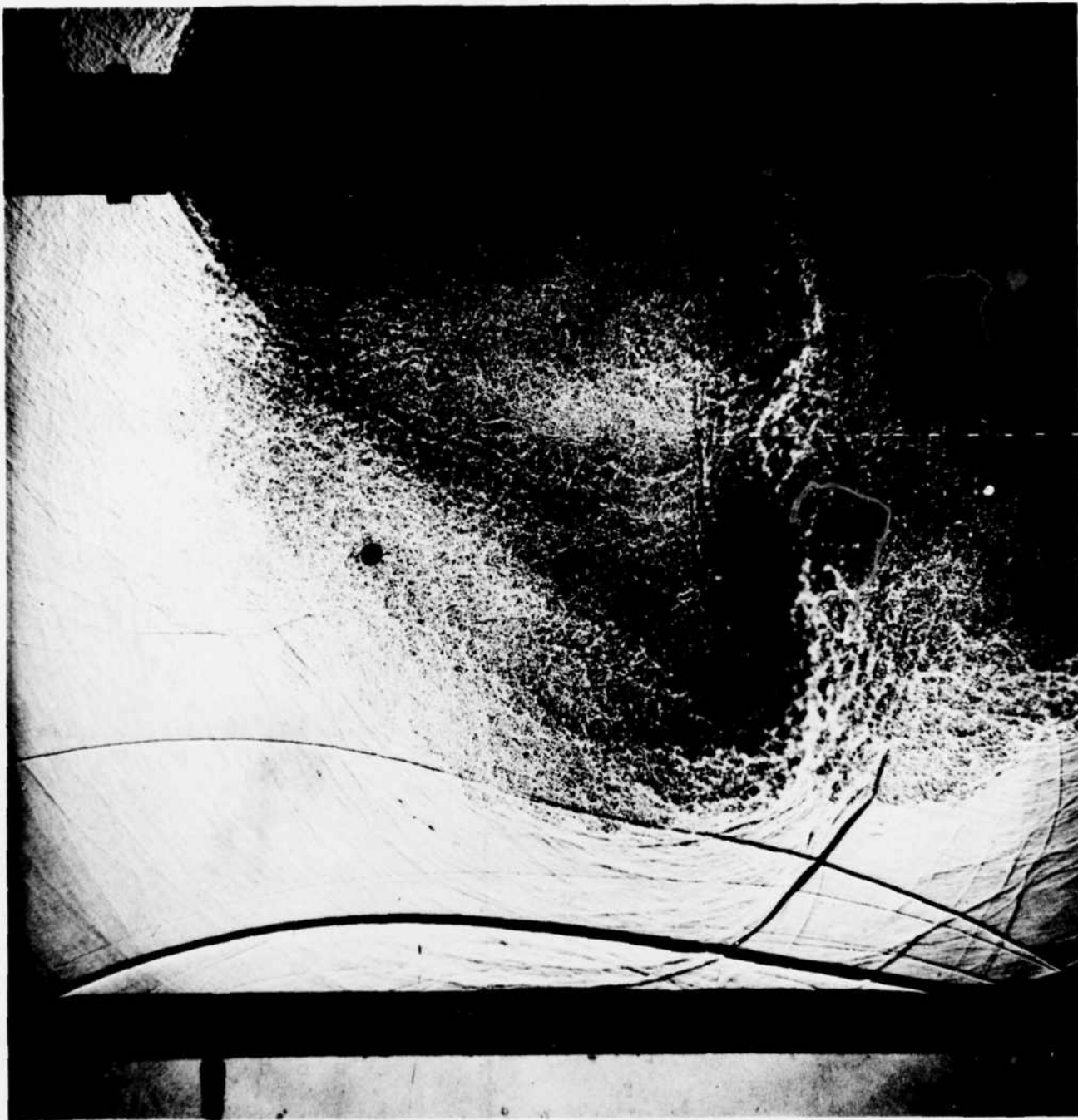
Figure 11. Spark Shadowgraph of Muzzle Blast Impinging Upon Plate Surface
