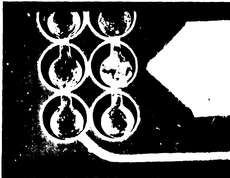
FIGURE 30. Laminar RM (IPC-B-25). Unsolderable Pad Due to Solder Mask Debris.
