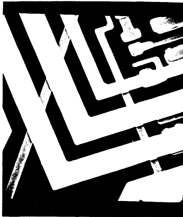
Fig. 3.3-2 Photomicrographs of portions of circuits on wafer showing second layer metallization lines fabricated using ion milling.
