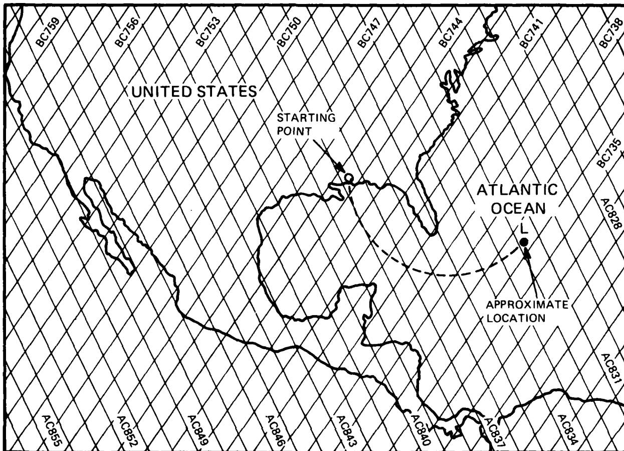
Figure 15. Lane Identification Based on Known Starting Point
