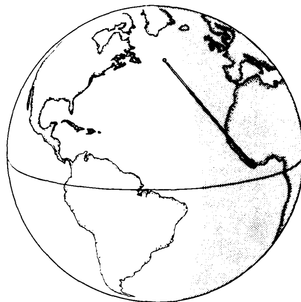
RECEIVER: N. ATLANTIC TRANSMITTER: LIBERIA NORTH-SOUTH PATH: SHORTER TRANSITION INTERVAL: LESS FIX ACCURACY
