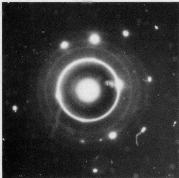
FIGURE 1. Selected area diffraction pattern obtained from the intercellular "S" phase.
