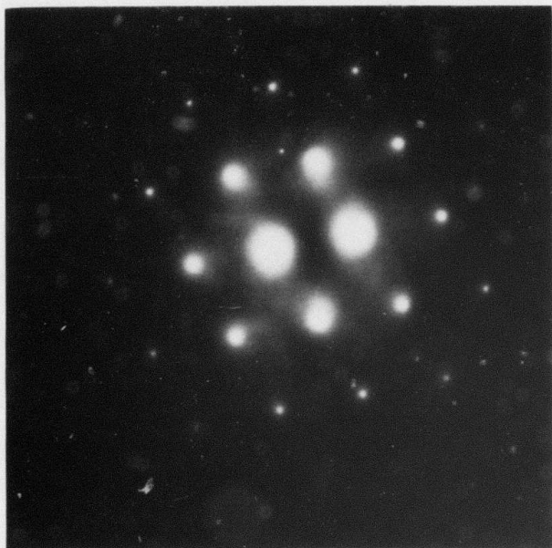
FIGURE 13. Selected area diffraction pattern which shows no evidence of the small quantity of "S" phase at the cell boundary of the A \lambda -1 wt. % Fe.
