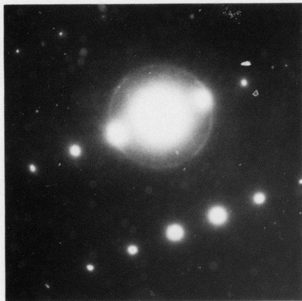
FIGURE 17. Al-3 wt. % Fe. Selected area diffraction pattern from the region shown in Figure 16. Note that diffraction ring originated from the cell boundaries.
