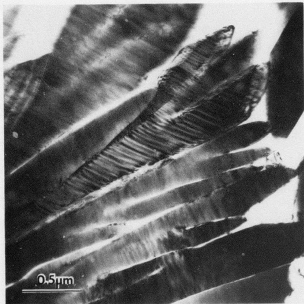
FIGURE 29. Al-34 wt.% Fe. Al_3Fe is the only phase detected in this alloy.
