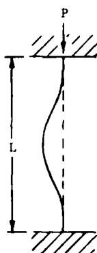
SHAPE OF NEUTRAL AXIS UNDER LONGITUDINAL LOADS
