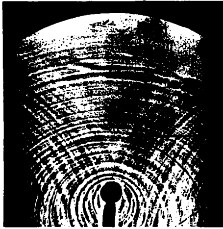
Figure 18. Shadow optical photograph of a propagating crack in steel.
