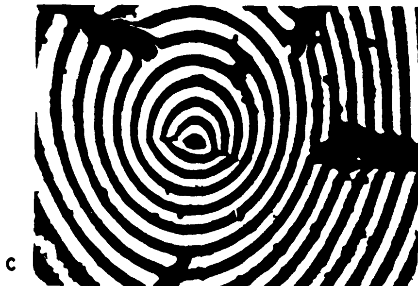
Figurella. Photomicrograph of a region of a cover slip/FM 1000/glass joint after immersion in distilled water for 40 hours at 60C b. Same as (a) with crossed polars
