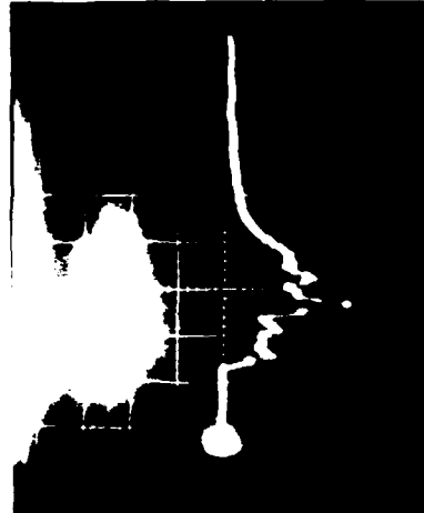
Figure 91. Transient record of discharge 11:41 on 0.03 cm solar cell cover glass exposed to 26 kV electron.
