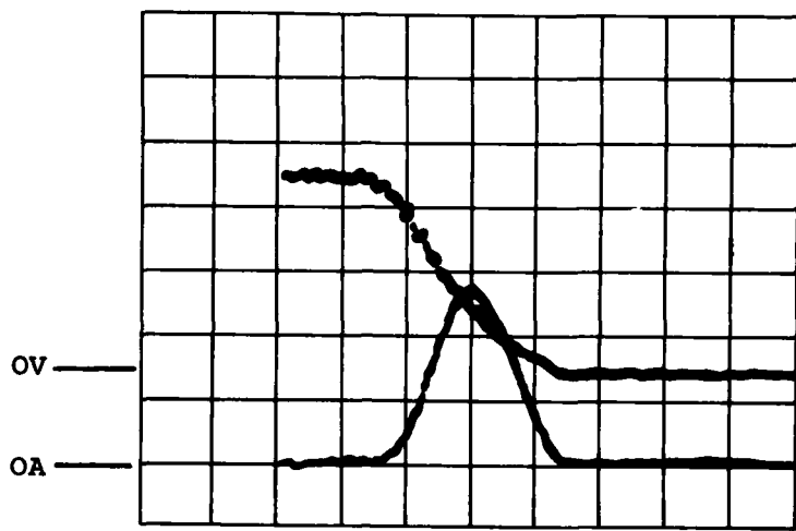
Figure 12. Typical Thyatron Commutation Waveforms With a Hot Cathode
