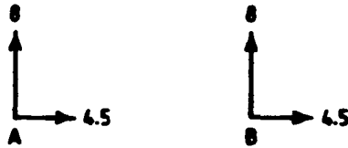
9 (b) Anchorage loads with equal strap tension
