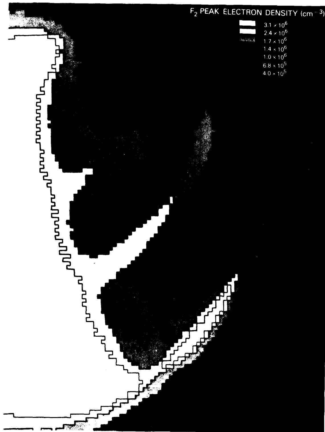
Fig. 9 — Contours of peak electron density (electrons cm -3 ) derived from the Apollo-16 photograph in Fig. 2. Note that the dayside image is overexposed.
