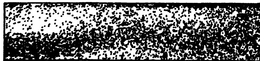
Fig. 8d. Powder concentration for 5 \mu\text{m} particles at 0.2 sec. Configuration h.
