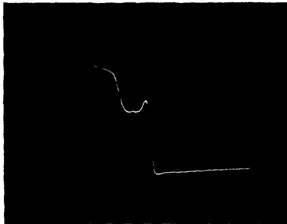
Fig 6 Oscilloscope trace of pressure distribution under tee seal
