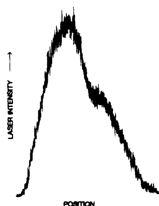
Fig. 4. Variation of UV laser light intensity across an approximately 3 mm diameter unfocused frequency doubled dye laser beam.
