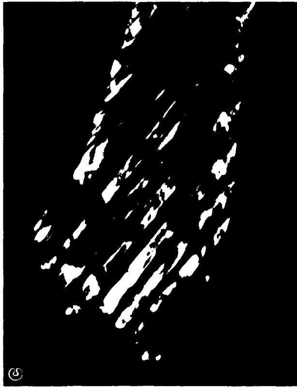
Figure 5. Al-rich martensite phase consisting of alternate twins in the boron-free ribbon.
