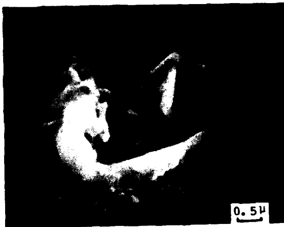
Figure 17. Single Impact Damage 1095 Steel Heat Treated to Maximum Hardness 90 Degree Impingement
