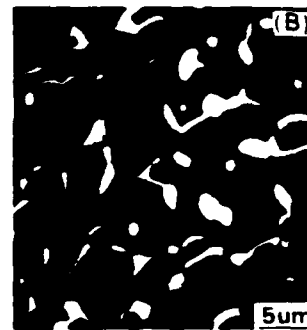
Fig. 4. (A) Diagram showing coalescence of inclusions at 4-grain junctions and (B) micrograph showing several \text{ZrO}_2 grains at 4-grain junctions resulting from coalescence (5 vol% \text{ZrO}_2 , 1700^\circ\text{C} for 2 h).
