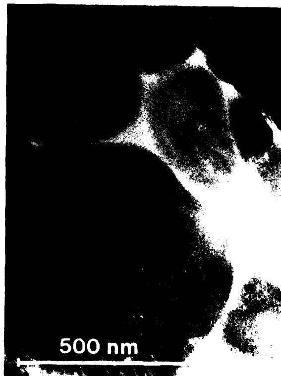
Fig. 4 a) Unmilled, sintered \text{ZrO}_2 (+ 2.3 m/o \text{Y}_2\text{O}_3 ) material (arrow points to crack), b) milled, sintered \text{ZrO}_2 (+ 2.3 m/o \text{Y}_2\text{O}_3 ). Both a) and b) show light and dark field images to indicate glass.
