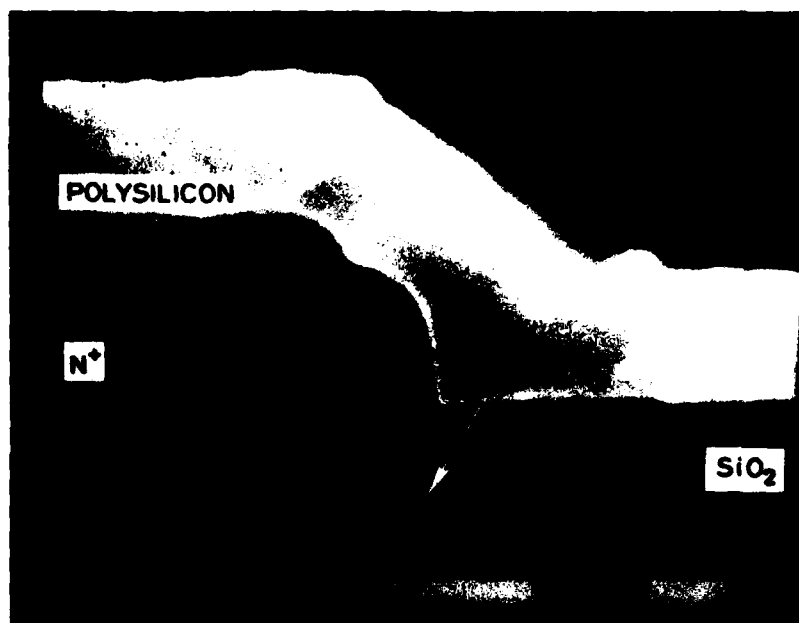
Figure 1-24: SEM cross-section of isolation structure with the smallest fabricated interface radius. r = 0.57 \mu\text{m} .
