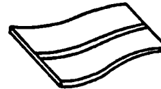
(f) BUCKLING DISTORTION
