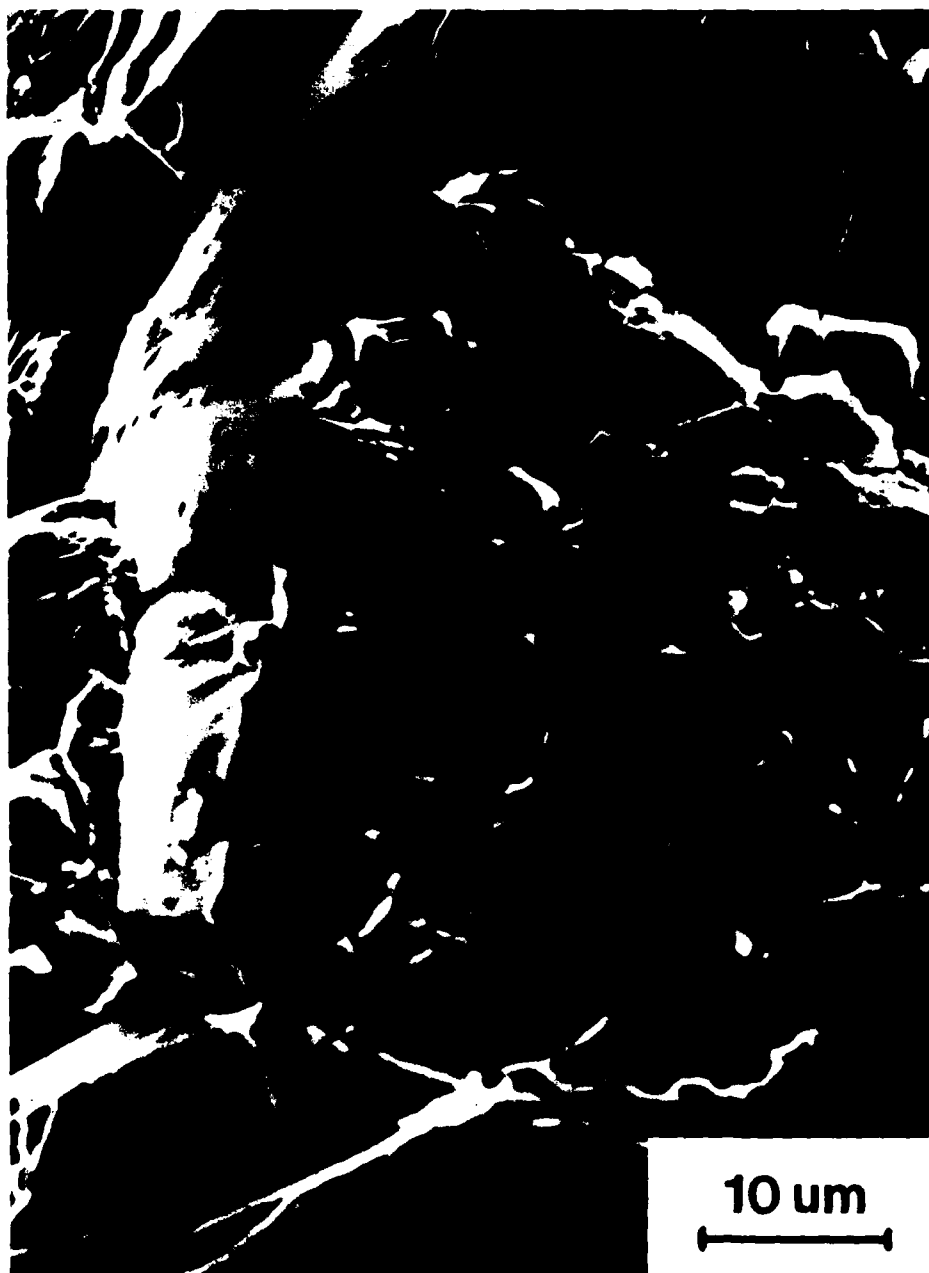
Figure 2. Shear bands, seen as narrow or broad white bands, on the bent tensile surface of \text{Ni}_{75}\text{Si}_8\text{B}_{17} glass ribbon material stiffened and strengthened with 5 volume percent of TiC particles.
