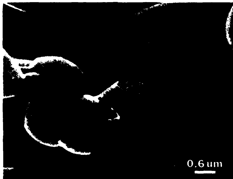
Figure 7.17 Fracture surface of \text{ZnO} with 1 m/o \text{Al}_2\text{O}_3 addition fired in hydrogen at 1100^\circ\text{C} for 60 minutes showing second phase of \text{ZnAl}_2\text{O}_4 at grain boundaries (arrow).
