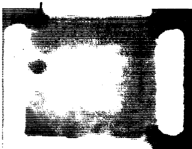
Figure 8. Through-Transmission of Al/Epoxy/Al Sandwich. Heavily corroded inner surface is not detected. Varying degrees of lightness are due to varying thickness of epoxy layer. Supports holding sandwich are seen on left and right sides.
