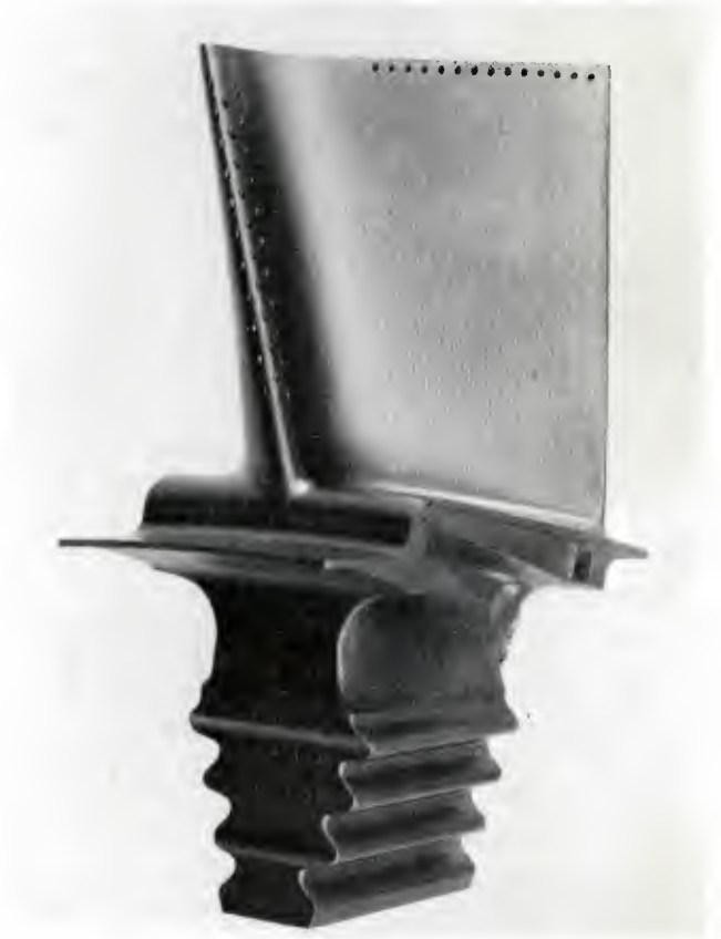
FIGURE 20 Turbine blades and vanes of a PW2037 engine (courtesy of United Technologies Corporation, Pratt and Whitney Aircraft).
