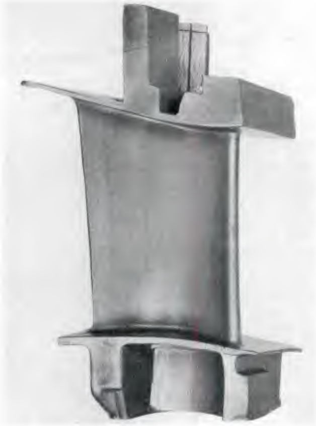
FIGURE 20 Turbine blades and vanes of a PW2037 engine (courtesy of United Technologies Corporation, Pratt and Whitney Aircraft).
