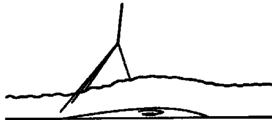
a. Shock parallel to leading edge on infinite yawed surface
