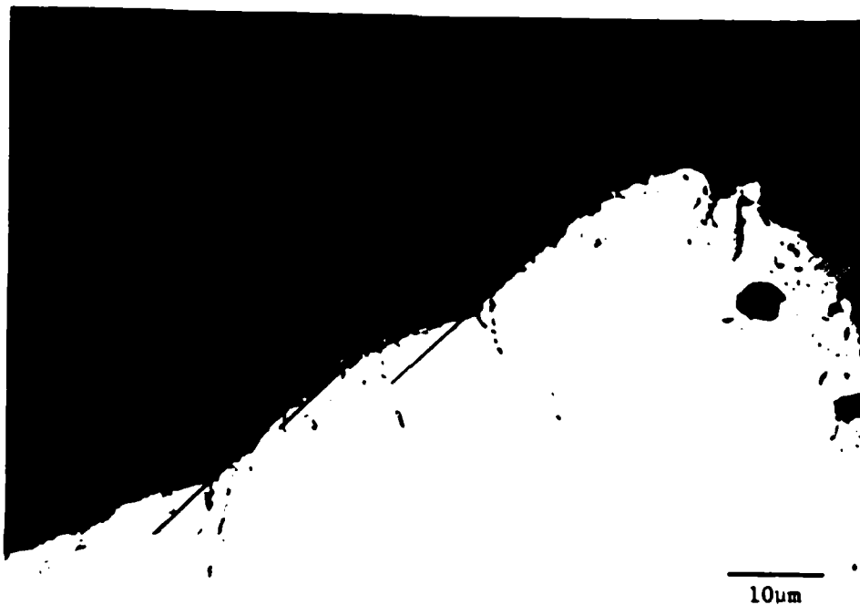
Figure 8. (a) Cross-sectional view of fracture surface shown in Figure 7. The black lines indicate the (111) fracture planes between the environmentally affected cleavage-like surfaces.
