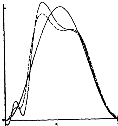
Fig. 85. Results for test-case 4: —, exact solution; — —, Lax-Wendroff; - · - ·, scheme 4. (Ref. 222)
