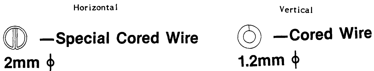
Figure 5. Flux Cored Wires for Out-of-position Welding by the GMAW-NG Process. Sumitomo Metal Industries Catalog.
