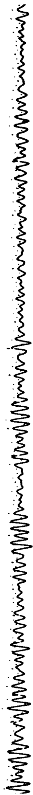
MODEL 44000Z - FLAT ACCELERATION, 0.001 Hz TO 4.0 Hz MAGNIFICATION \approx 10K AT 25 SECONDS
