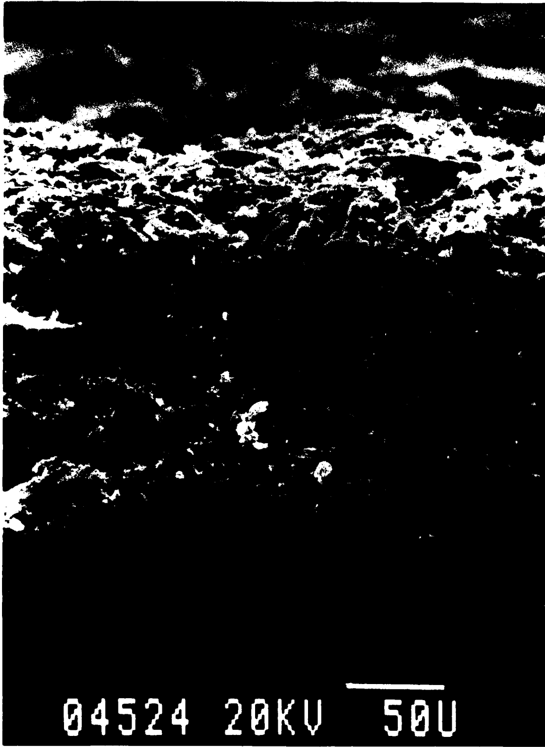
Figure 6: Scanning Electron Microscope Photograph of a Cross-section of Paper Containing Activated Carbon.
