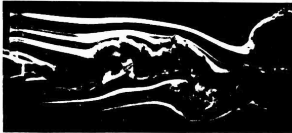
Figure 1. Smoke flow visualization of a fluidically oscillating jet.
