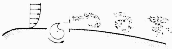
Figure 5a. Schematic of vortex generation in the upper surface of an airfoil.
