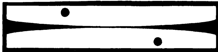
Figure 21. Ka band waveguide to fin-line 2 \lambda transition mask ( 2:1 scale ).
