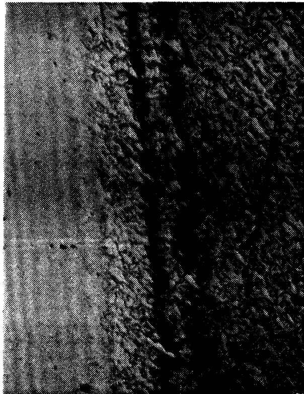
Figure 22. Angle lapped sample of \text{SiO}_2/\beta\text{-SiC/Si} at a 36^\circ angle to produce a magnification of 100X. The magnification of the photographic 400X. The dark bands are color fringes in the oxide. The actual oxide/SiC interface is not visible because the SiC does not provide sufficient reflectance to show this interface.
