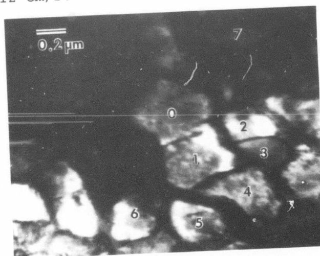
FIGURE 5. STEM micrograph of cellular structure solidified at 18 cm/s. The compositions at the centers of the cells marked 0, 1, ... 7 respectively are 12.5, 13.0, 13.8, 15.5, 14.8, 13.8, 12.0, 13.2 wt% Cu.
