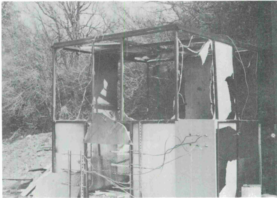
Figure A-16. Damaged Cube After Test 22
