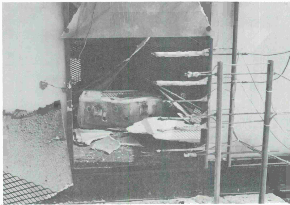
Figure A-17. Vented Ammunition Box Used to Contain the Four Flares
