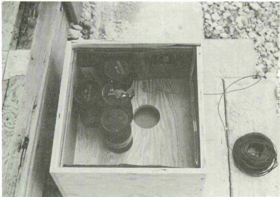
Figure 19. Center Grenade Wired for Remote Actuation
