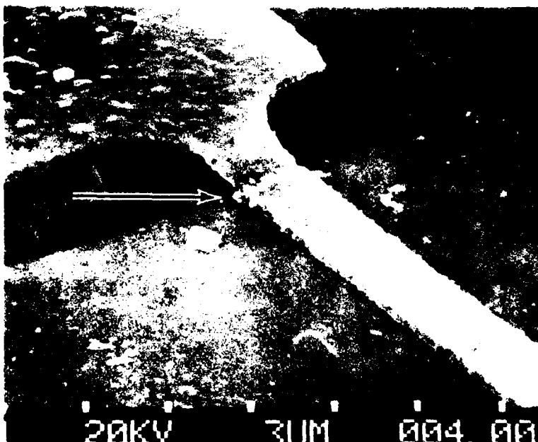
Figure V.H.37 - CD Stress, Pin 5 Polysilicon Breakdown Site
