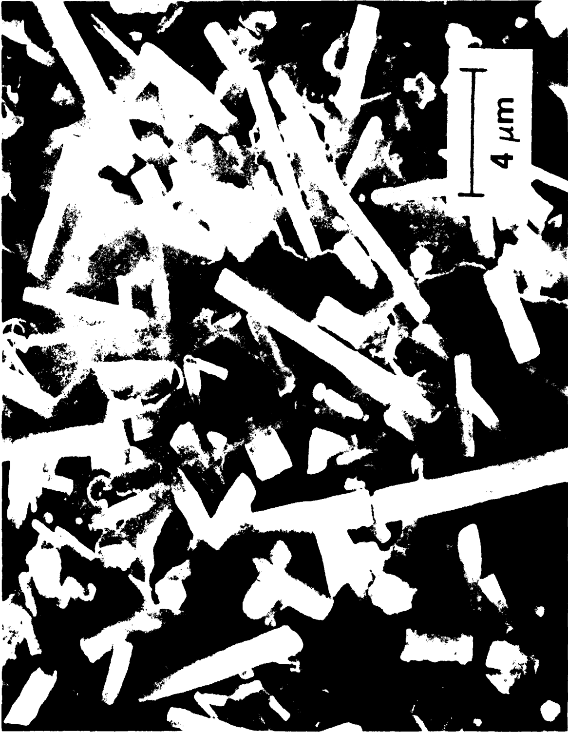
Fig. 2 - Micrograph of 20V/o F-9 SiC/6061-T6 aluminum metal matrix composites
