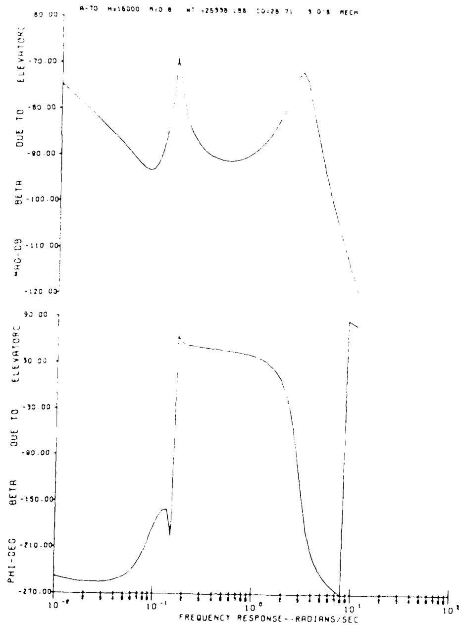
Figure F39. 3G Mechanical Bode Plot for Beta due to Pilot Elevator Input.
