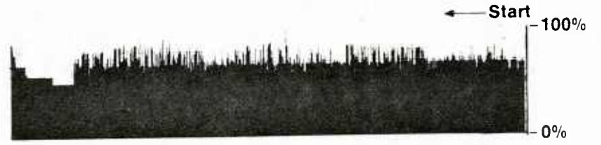
(C) Compressive Loads Truncated (GAR 1)
