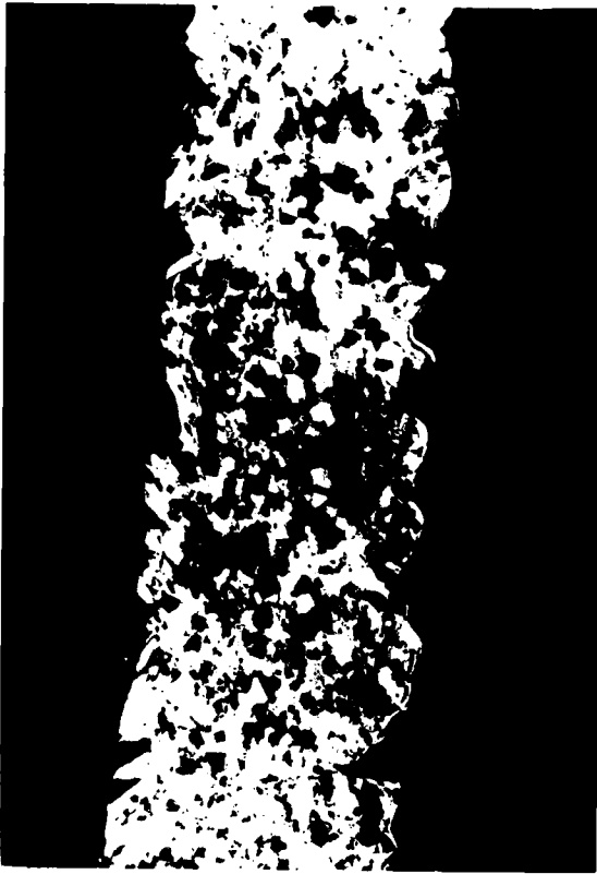
a. Ice-wedge ice, with only central, upper part of core appearing to be unaltered.
