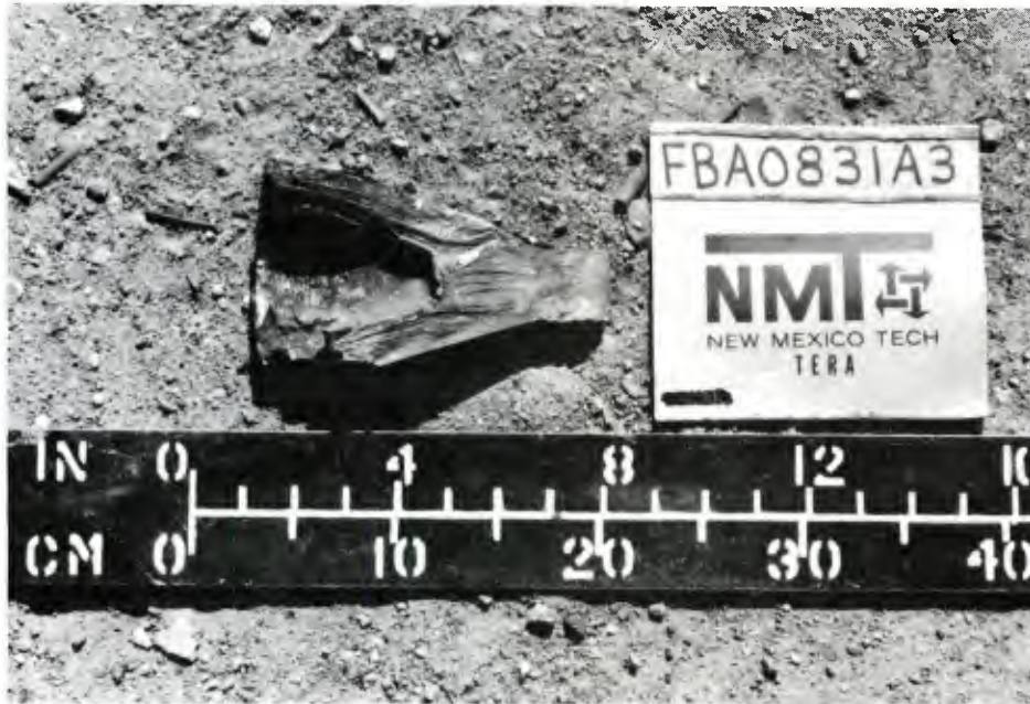
ACCEPTOR #1 - FUZE CAVITY FRAGMENT - AFTER TEST
