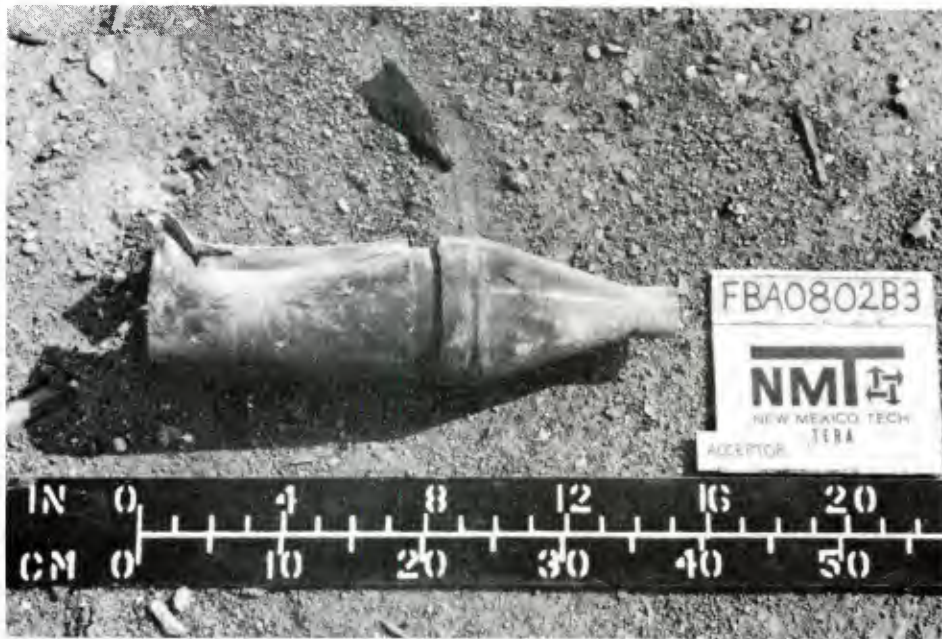
ACCEPTOR #2 - DAMAGED WARHEAD AND FUZE CAVITY AFTER TEST
