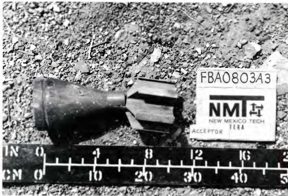
ACCEPTOR #2 - DAMAGED FUZE CAVITY AND TAILBOOM
