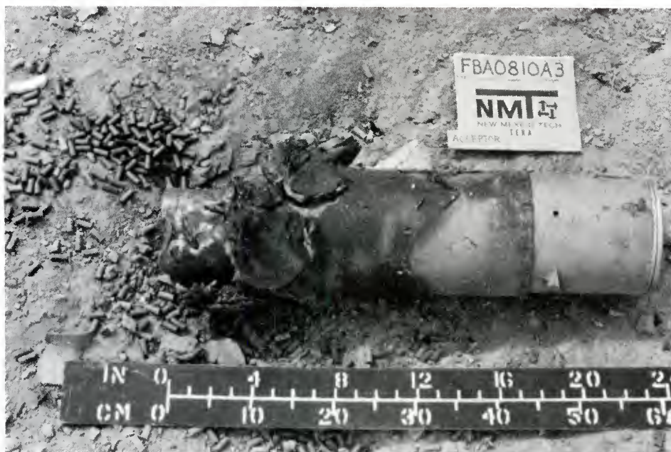
ACCEPTOR #1 - DAMAGED CARTRIDGE CASE AND SHIPPING TUBE AFTER TEST
