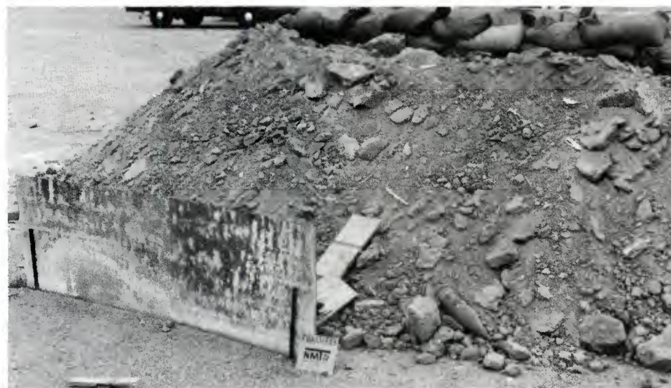
REAR VIEW SHOWING DEBRIS AND UNDAMAGED WITNESS PANEL AFTER TEST
