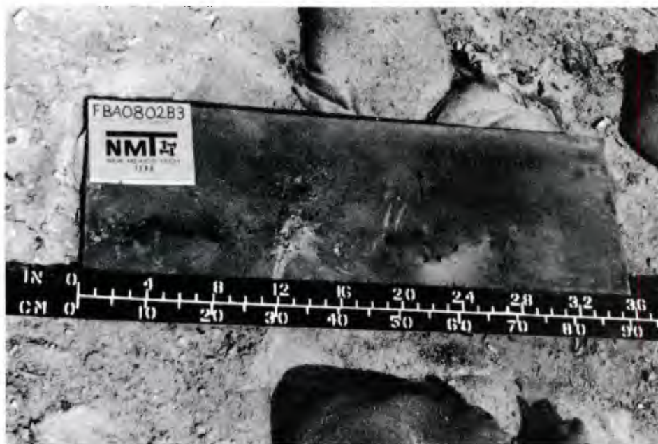
WITNESS PLATE - AFTER TEST ONLY APPARENT JET FORMATION WAS FROM DONOR PROJECTILE
