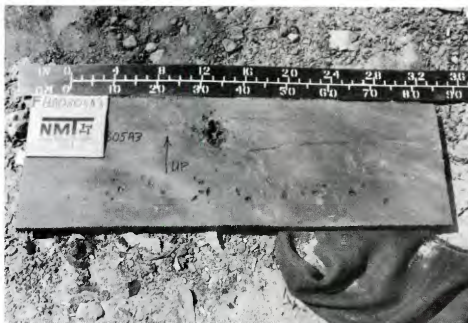
WITNESS PLATE - AFTER TEST ONLY APPARENT JET FORMATION WAS FROM DONOR PROJECTILE
