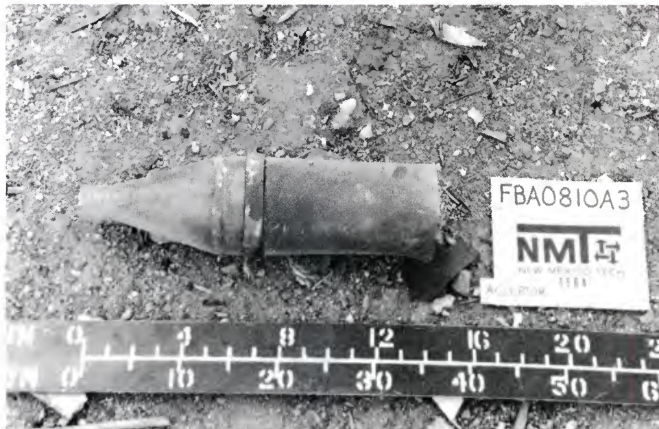
ACCEPTOR #1 - DAMAGED WARHEAD - AFTER TEST
