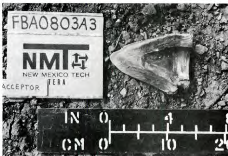
ACCEPTOR #1 - FUZE CAVITY FRAGMENT - AFTER TEST
