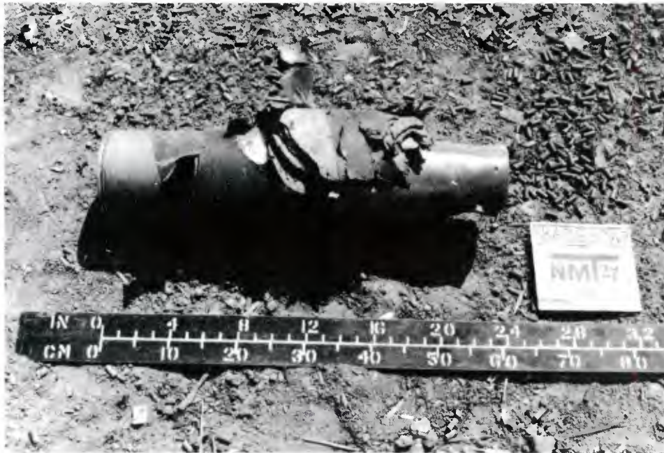
ACCEPTOR #2 - DAMAGED CARTRIDGE CASE AND SHIPPING TUBE AFTER TEST
