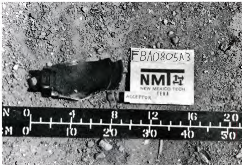
ACCEPTOR #1 - WARHEAD FRAGMENT - AFTER TEST
