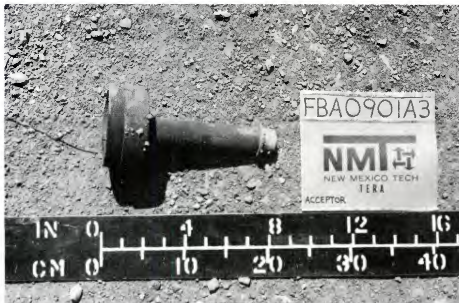
ACCEPTOR #2 - STANDOFF NOSE - AFTER TEST
