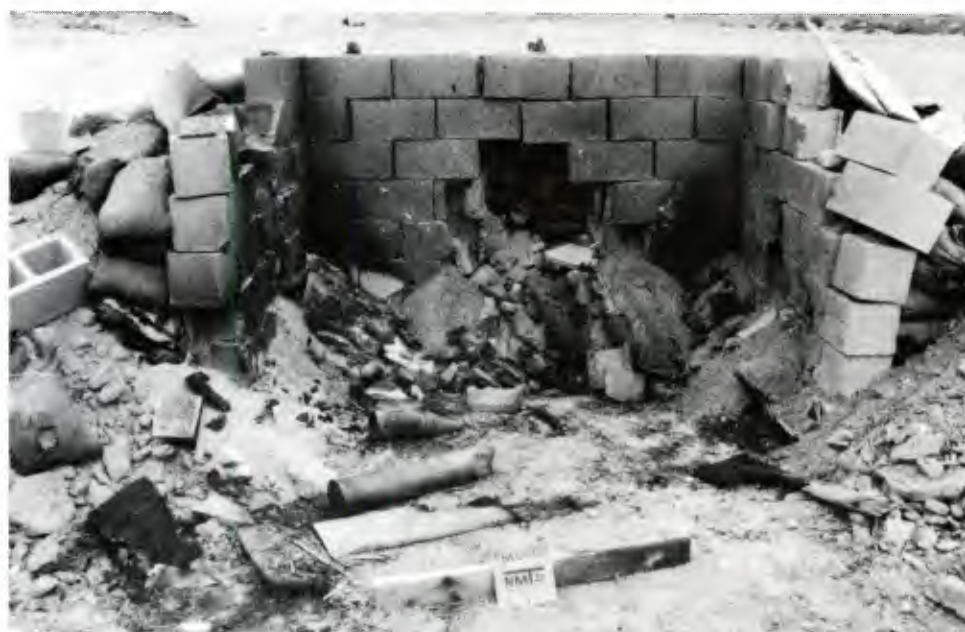
FRONT VIEW SHOWING DEBRIS AND DAMAGE TO STORAGE FACILITY AFTER TEST
