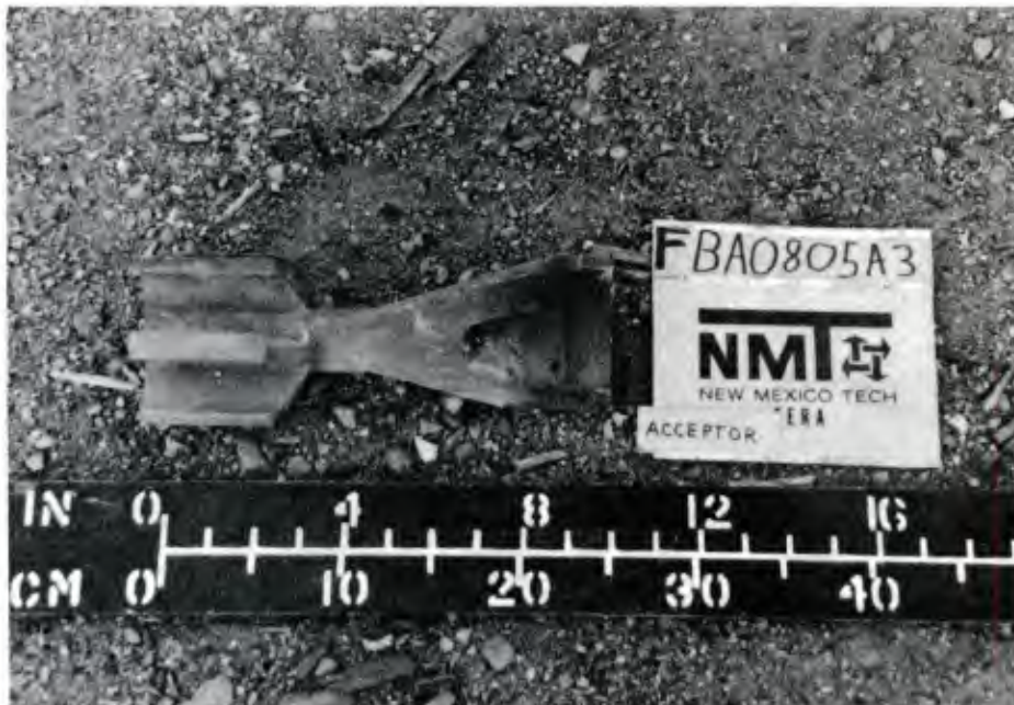
ACCEPTOR #1 - FUZE CAVITY AND TAILBOOM FRAGMENT AFTER TEST
