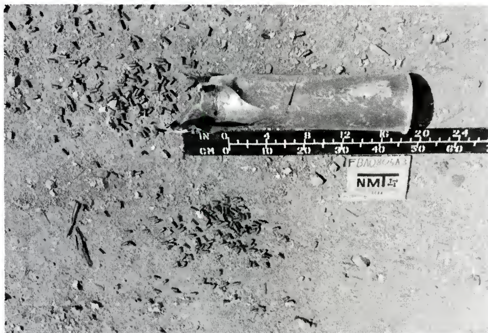
ACCEPTOR #2 - DAMAGED CARTRIDGE CASE AFTER TEST
