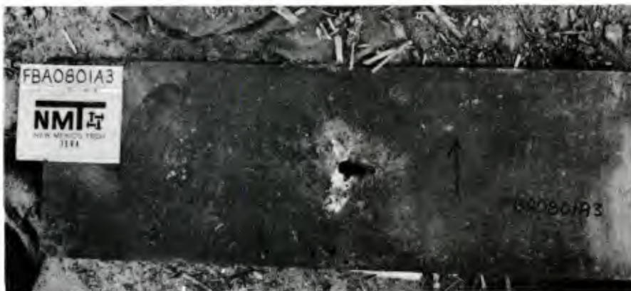
WITNESS PLATE - AFTER TEST ONLY APPARENT JET FORMATION WAS FROM DONOR PROJECTILE
