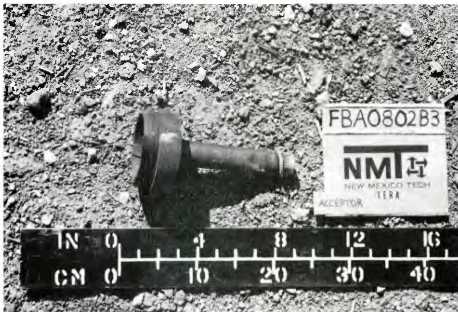
ACCEPTOR #1 - STANDOFF NOSE - AFTER TEST
