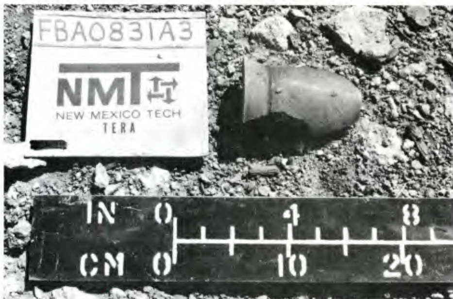
ACCEPTOR #1 - WARHEAD FRAGMENT - AFTER TEST
