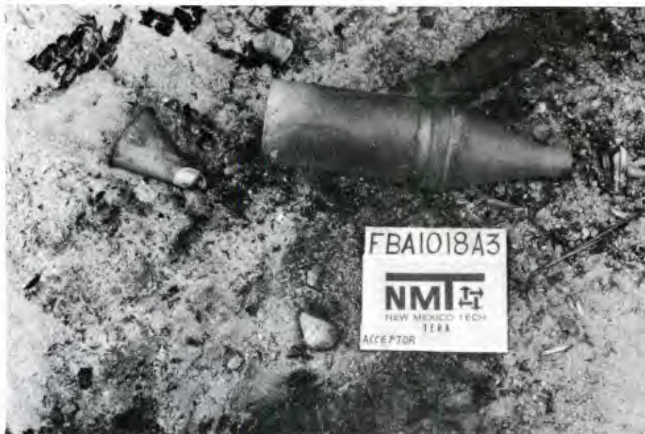
ACCEPTOR #L-1 - DAMAGED WARHEAD - AFTER TEST
