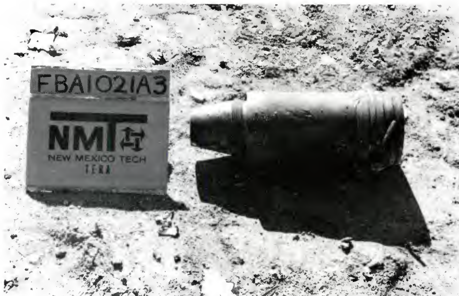
K.E. ROUNDS - PROJECTILES SHOWING TYPICAL POST-TEST DAMAGE
