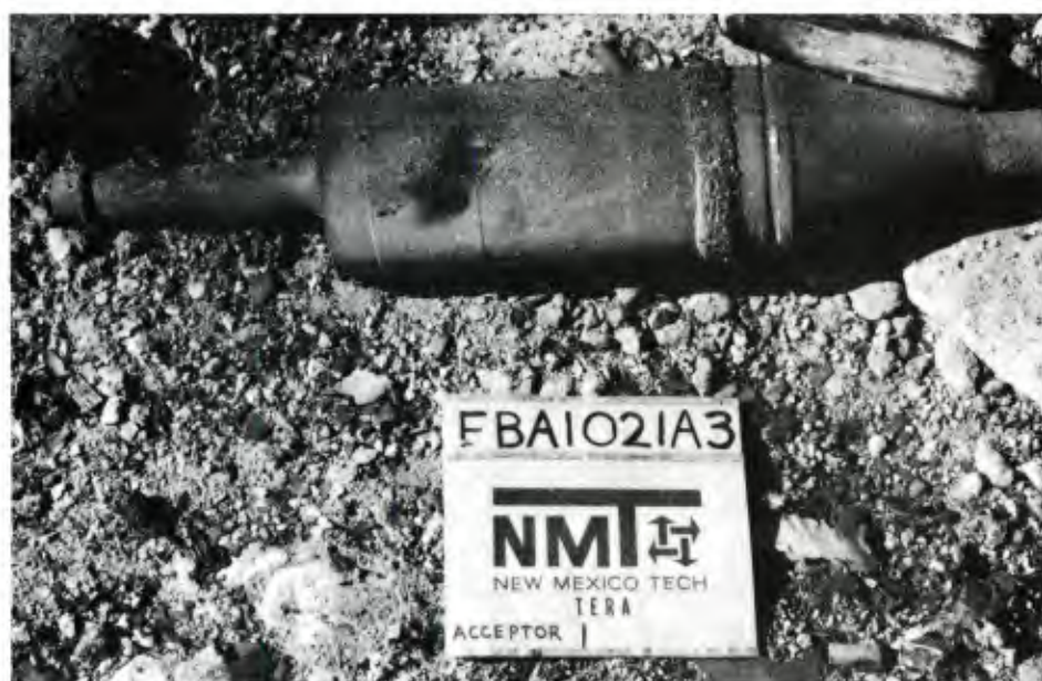
ACCEPTOR #L-2 - DAMAGED WARHEAD - AFTER TEST
