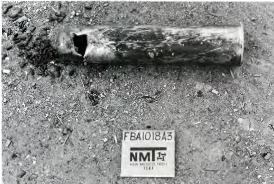
ACCEPTOR #L-1 - DAMAGED CARTRIDGE CASE - AFTER TEST
