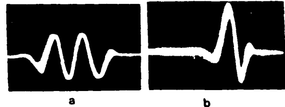
Fig.4 Coherent video signal during the transmitter pulse. a. 1 microsecond pulse. b. 300 ns pulse. Coho frequency offset is approximately 2 MHz.
