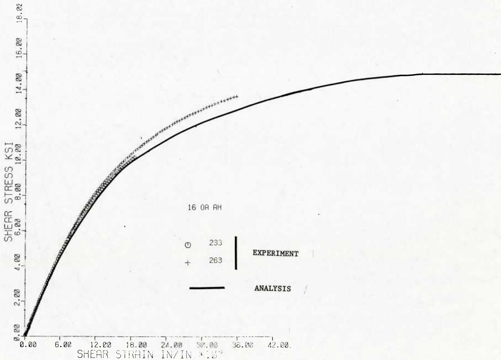
Figure 56. Shear Stress ( \tau_{12} ) versus Shear Strain ( \gamma_{12} ) Curves for 16° Off-axis Specimens with Square Tabs and Hinged Grips
