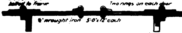
DETAIL OF M.H. FRAME AND COVER This ironwork to be furnished by City and set by Contractor. Scale: 3" = 1'
