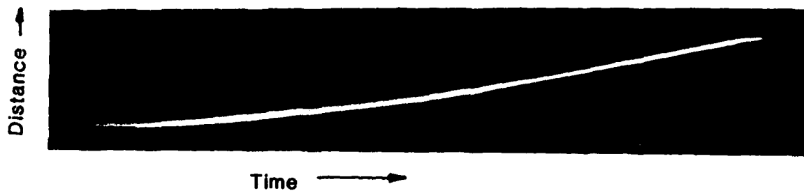
Figure 1. Streak photograph for firing RPIP 02. In Figs 1 & 2 the horizontal scale is approximately 1\text{mm} \equiv 5.5 \mu\text{s} and the vertical scale approximately 1\text{mm} \equiv 22 \text{mm} .
