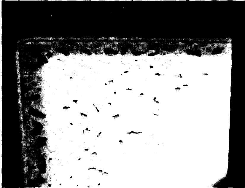
Figure 14. Bond Pad Area on Sample 22-9 (Hydrogen Doped).
