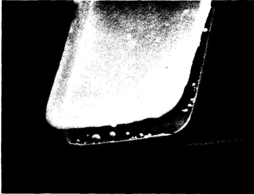
Figure 8. SEM Photograph of Lifted Contact Pad on Failed Circuit.
