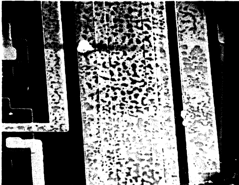
Figure 12. Gross Voiding on Sample 22-9 (Hydrogen Doped).
