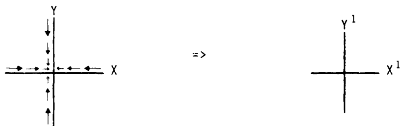
Figure 2.3.a. Convergence ( \partial u/\partial x + \partial v/\partial y negative, horizontal area decreases)
