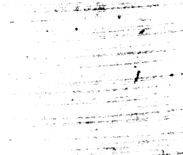
Figure 45. Striation etch pattern for non-rotating section of crystal Z322 grown with magnet off.
