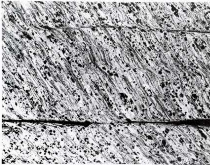
FIGURE 12. Plug Fragmentation Along an Inhomogeneous Shear Band. (2024-T4 Aluminum, 100X magnification.)
